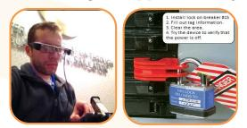
A senior design project developed an app for both the Epson Moverio and the Google Glass devices that allow users to access a library of step-by-step instructions of lock out/tag out procedures using the head mounted device (HMD) that ensures the lock out or tag out is completed properly and in the safest way possible.
